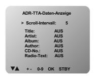
In the first menu entry, the scroll interval time of the TTA data records in the LED display is set. This is adjustable between 1+5 steps.
